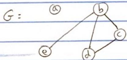
$$\begin{array}{ll} \deg(a) = 0 & \deg(d) = 2 \\ \deg(b) = 3 & \deg(e) = 1 \\ \deg(c) = 2 & \end{array}$$
